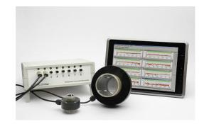
Real-time permanent biosensing with the biomonitor monitors the toxic risk of chemical mixtures on indicator organisms, recorded as stress behaviour (ventilation, avoidance, morbidity) and mortality. Both, acute effects of pollution peaks due to accidents and spills, and chronic effects of low-dose substances can be detected immediately and actions triggered (water sample for diagnostic analytics).
