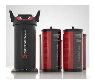
Demineralisation device with replaceable cartridge. For initial filling and circuit desalination. Integral meter. Wireless transmitter for automatic shut-off of external devices, such as pumps and solenoid valves. Wireless plug (receiver) available as an option. The PUROTAP HIGHPOWER or PUROTAP NEXION replaceable cartridge can be simply and cleanly inserted into the device.
