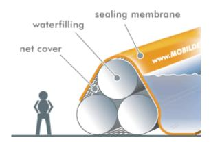
The **Mobildeich** consists of individual dyke elements that are available in different sizes and lengths. You can use the modules in any combination with each other and connect them to a stable chain of dykes.
