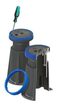
Experience has taught us that road damage may occur when no proper joint is formed between surface box and tarmac road surface. The surface box with so called "Fugenring" offers the perfect solution to avoid this potential problem.
