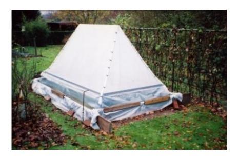
Equipment for the production of pure H2O for drinking water from sea, river and brackish water using solar energy.
